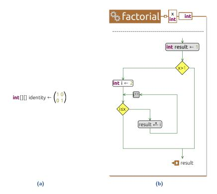
Figure 6.1: Different visual notations in Envision: (a) textual (declaration of identity), mathematical (matrix initialization); and (b) graphical.
