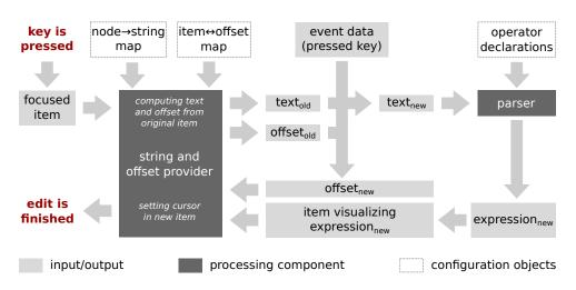
Figure 6.8: The process of editing an expression after a key has been pressed.
