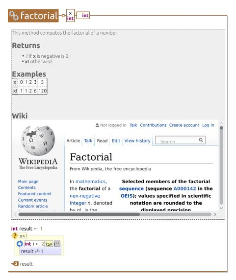
Figure 2.13: The factorial method with a rich comment header that includes rich text-formatting, a table, and an embedded browser.
