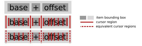
Figure 6.3: Four visual items representing the expression <code>base+offset</code> wrapped in a container. Top: the items' bounding boxes; middle: cursor regions without equivalent regions; bottom: cursor regions with equivalent regions.
