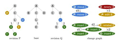
Figure 7.5: A base tree with two modifying revisions and the corresponding CG. Each edge in the CG is labeled with the dependency or conflict type that the edge represents.
