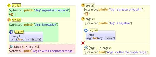
Figure 5.9: An if-statement  $(\diamondsuit)$  with an else-if  $(\diamondsuit)$  and else branches  $(\varkappa)$  in an early (left) and the current (right) Envision visual design.
