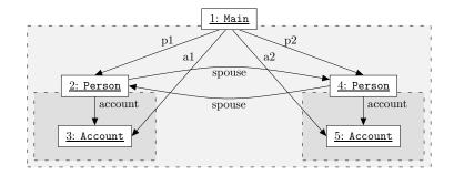
Fig. 1: Example of an ownership structure. Boxes and arrows depict objects and references, respectively. Dashed boxes enclose the objects of an ownership context; the owner of these objects sits atop the dashed box.
