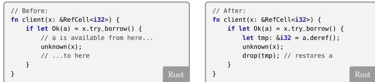
Figure 4.16: Example of a refactoring that introduces a conversion method call, a.deref() , using a place that was available across the unknown(x) statement.
